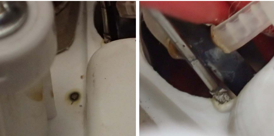
Figure 13 – Position of the nichrome wire and the results of the test.
