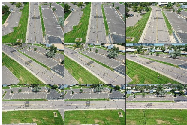
FIGURE 18 Drone Aerial Photographs- Top to Bottom 0°,45°,90° - Left to Right Incident angles: 30°,45°,70°
